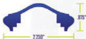
DIXIE CAP 2-1/4" X 7/8" ACCEPTS 1", 1-1/4" & 1-1/2" CHANNELS WT/FT: 0.670#
